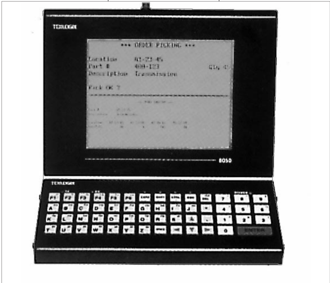
Figure 2 Truck Mounted Terminal (Teklogix 8050)
